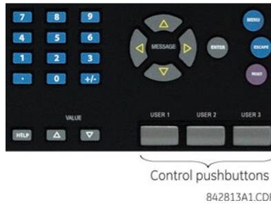
An additional four control pushbuttons are included on the standard faceplate when the C30 is ordered with the 12 user-programmable pushbutton option.
