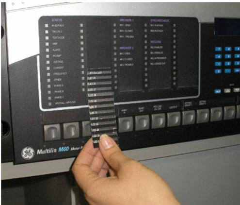
To remove the user-programmable pushbutton labels from the C30 enhanced front panel and insert the custom labels:
