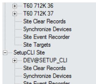
The device is named as DEV@SETUP\_CLI, which is used as the device name required by the <device> parameter of other SetupCLI commands.
