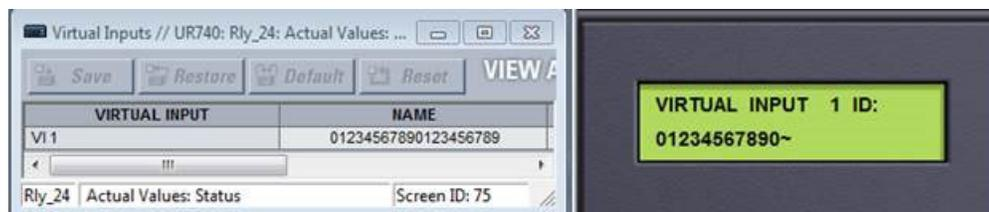
The front panel can be viewed and used in the EnerVista software, for example to view an error message displayed on the front panel.
