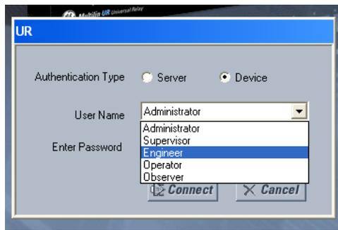
When the "Server" **Authentication Type** is selected, the C30 uses the RADIUS server and not its local authentication database to authenticate the user.
