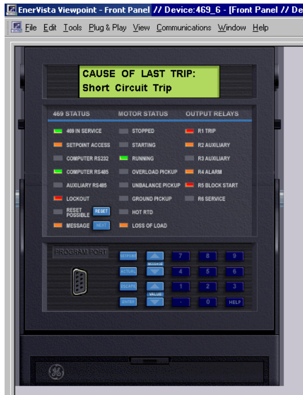
Figure 81: Controlling a device in Viewpoint Monitoring
