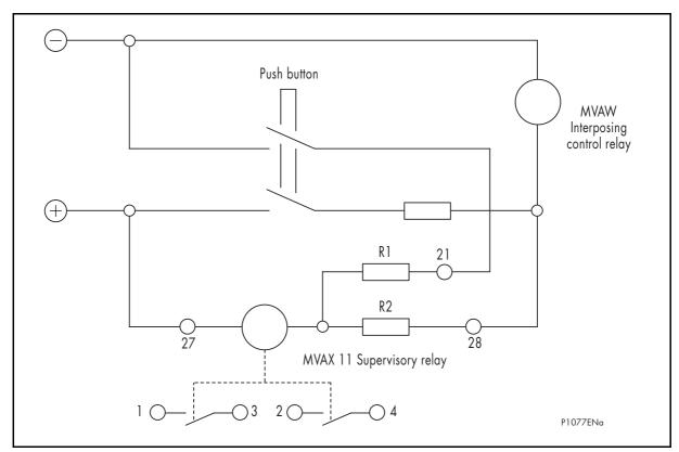
Figure 2: Supervision of interposing control relay type MVAW
