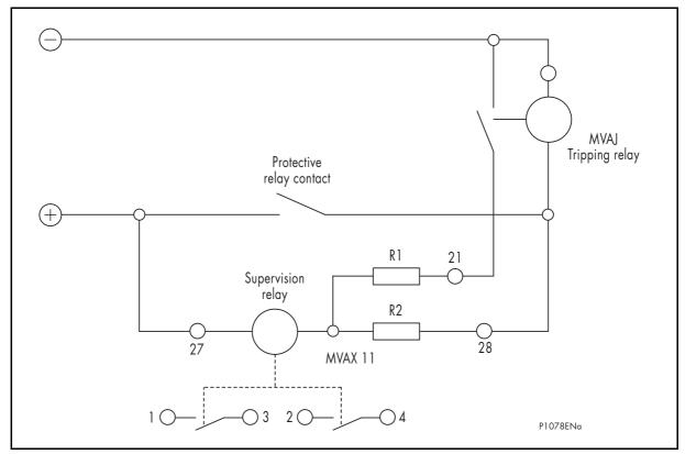
Figure 3: Supervision of tripping relay type MVAJ
