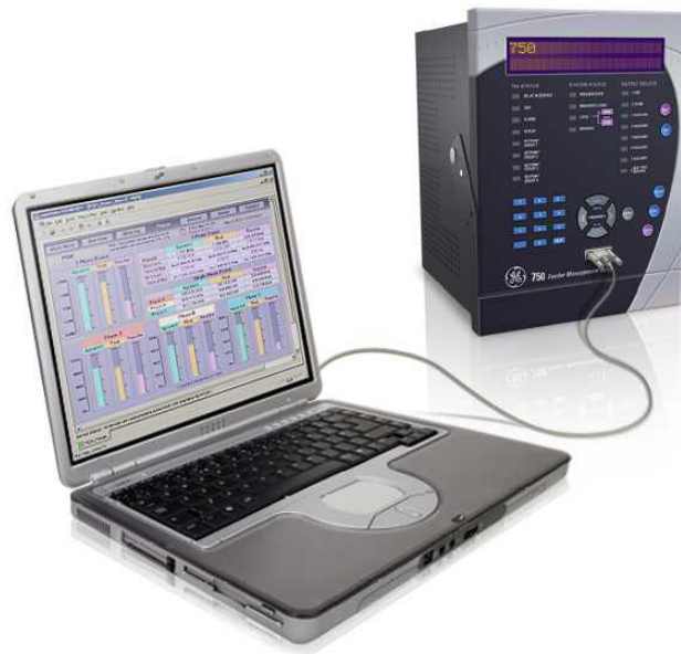
FIGURE 4-3: Communications using the Front RS232 Port
