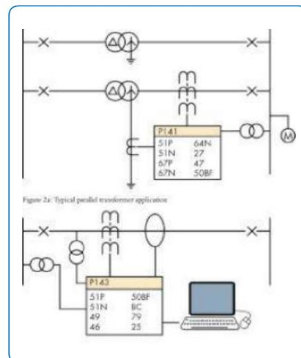
Figure 2a: Typical parallel transformer application
