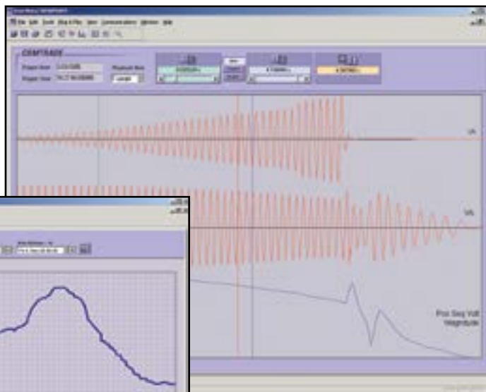
Analyze generator faults using both analog and digital power system quantities that are measured and recorded up to a rate of 64 samples per cycle.
